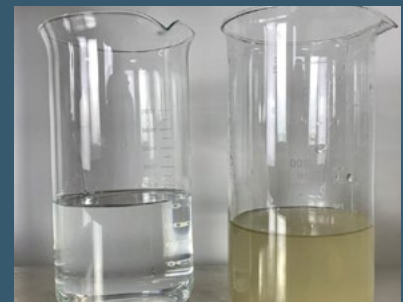
River water after passing through a sand filter
