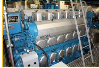
TMS Rudolf Deymann • Main engine: Wärtsilä 6L20 • 1.076 kW • Tanker • 110 m • 2.322 to.
