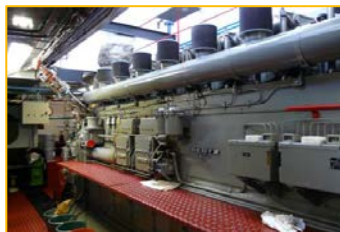
MS Empresa • Main engine: Deutz 545 • 745 kW • Dry cargo ship • 86 m • 1.500 to.
