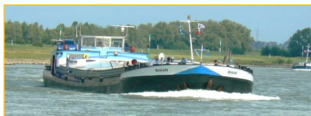
MS Mainland • Main engine: Deutz 628 • 883 kW • Dry cargo ship • 85 m • 1.516 to.
