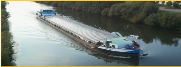
MS Coburg • Main engine: MWM TBD 440 • 720 kW • Dry cargo ship • 86 m • 1.724 to.
