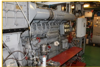
MS Coburg • Main engine: MWM TBD 440 • 720 kW • Dry cargo ship • 86 m • 1.724 to.
