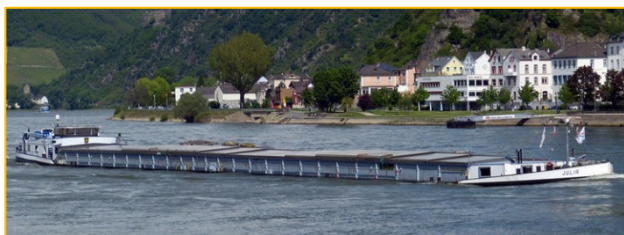
MS Julia • Main engine: Deutz 816 • 826 kW • Dry cargo ship • 105 m • 2.199 to.
