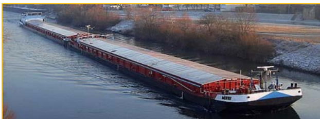
KV Heinz Hofmann • Main engine: ABC MDZC-166 A • 1.325 kW • Dry cargo ship • 186 m • 4.788 to.
