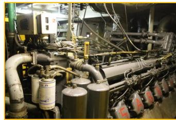
MS Julia • Main engine: Deutz 816 • 826 kW • Dry cargo ship • 105 m • 2.199 to.
