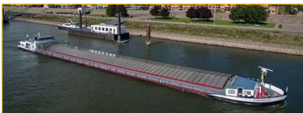
MS Empresa • Main engine: Deutz 545 • 745 kW • Dry cargo ship • 86 m • 1.500 to.
