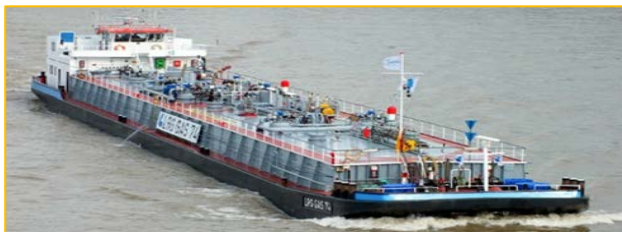
Imperial GAS 74 • Main engine: 2 x Mitsubishi • 634 kW • Tanker • 85 m • 1.158 to.
