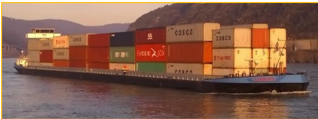
MS Aarburg • Main engine: ABC MDZC-166 A • 1.325 kW • Container Ship • 135 m • 3.297 to.
