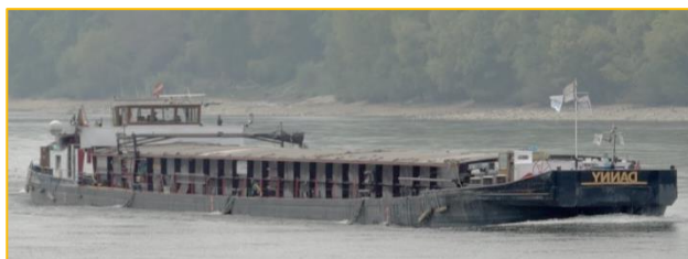
MS Danny • Main engine: Deutz 545 • 735 kW • Dry cargo ship • 85 m • 1.346 to.
